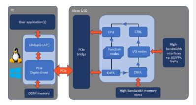
To address this, TOPIC developed Dyplo®, a Dynamic Process Loader. On the FPGA side, Dyplo® forms a Network-on-Chip (NOC), wrapping fixed and dynamically exchangeable FPGA function blocks. On the processor side, Dyplo® is a Linux kernel driver/API that interfaces with the Dyplo® NOC using file based data streams. The third aspect of Dyplo® is the implementation flow to transform a software defined function block into a Dyplo® wrapped FPGA function block.
