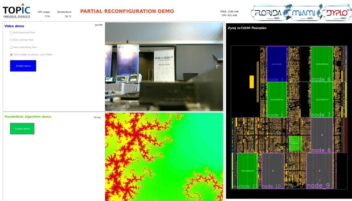
Figure 6 – A Qt-based example application running 2 applications simultaneously in the NOC
